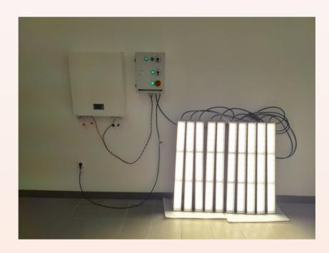
The same lighting fixture works both as a standard LED light on AC power 230V / 50Hz at 100% luminous flux intensity and in case of loss of power, the same LED light begins working as an emergency light at approximately 15% luminous flux intensity through the emergency controlling box and the LiFePO4 battery on DC 48V.
